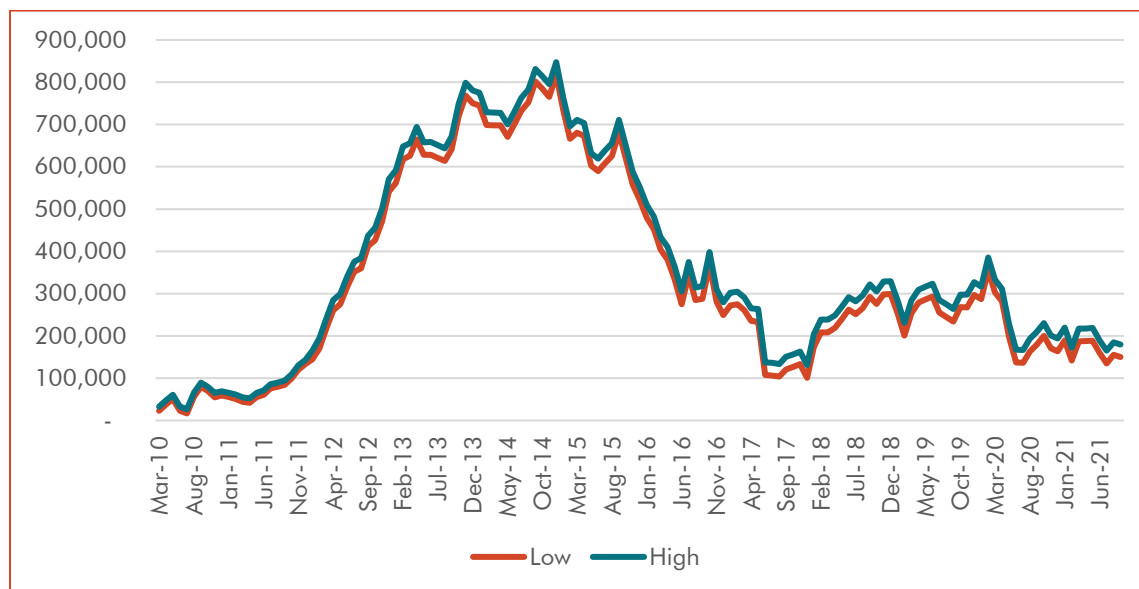
Figure 3-40: Barrels per Day of Crude Oil Shipped by Rail from North Dakota
