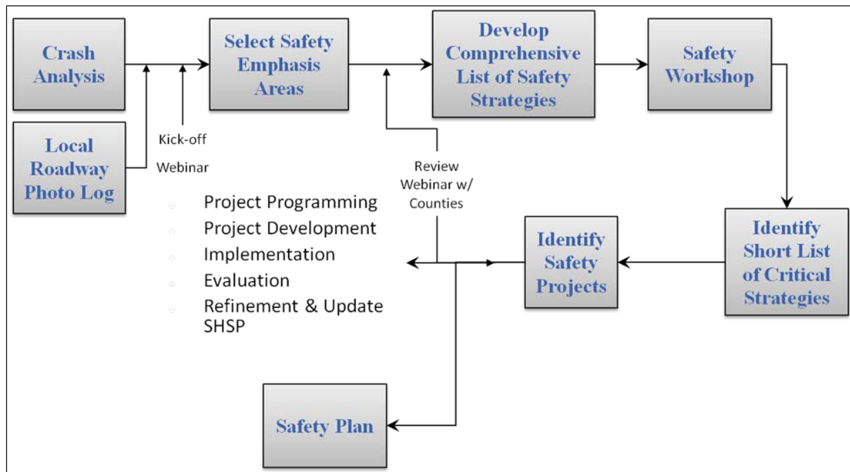
FIGURE 1-3 Local Road Safety Program Safety Plan Approach
